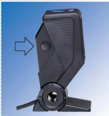
omnidirectional or single-line mode select button
